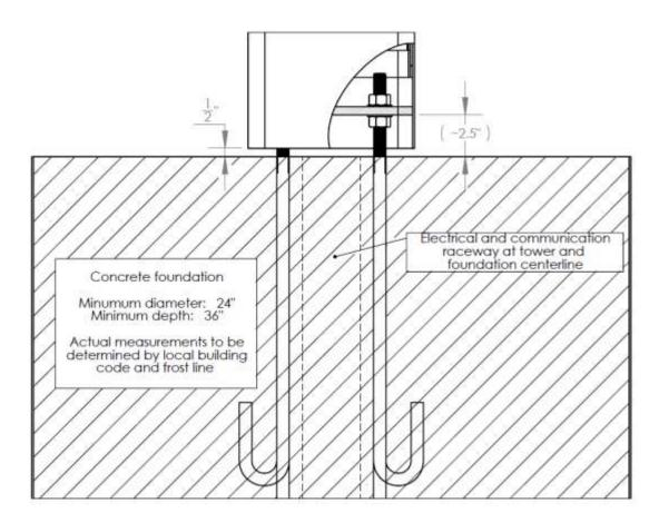
4. Install one 3/4" nut and one washer on each anchor bolt 2.5"-3.5" above grade to top of washer. This will allow for a <u>1/2" air gap</u> between the foundation and the Pedestal which will allow airflow and prevent moisture problems. Verify that the nuts are level (0° pitch).
