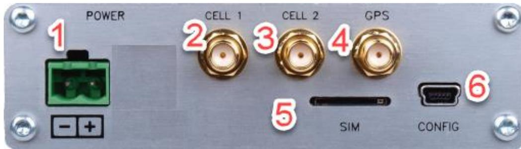
**Figure 3.** Rear panel of the **ETP-CI-4G-V** Cellular Interface.
